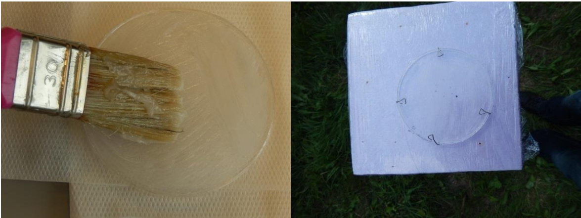
Fig S7. Spore trap based on 10 mm Petri dishes coated with a mix of Vaseline® and Paraffin wax®
