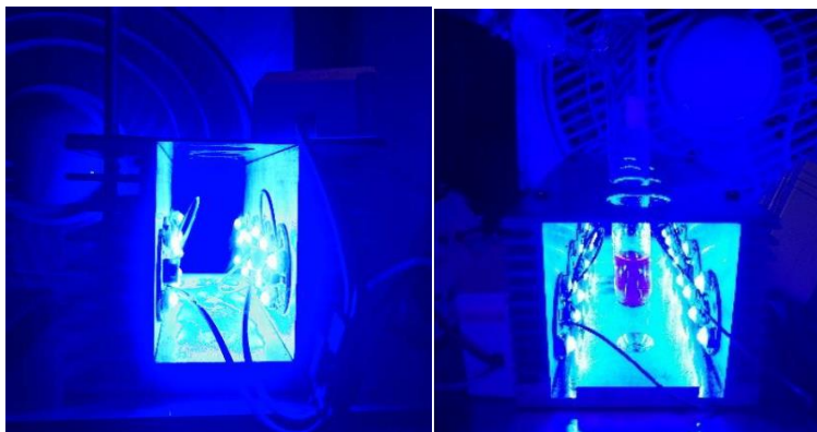
Supplementary Figure 1. The blue LEDs photochemical setup.
