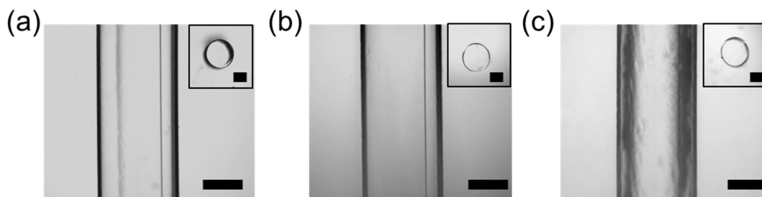
Figure S9. Hydrogel fiber expansions in different concentrations of glucose solutions. (a) 0 \text{mmol L}^{-1} , (b) 10 \text{mmol L}^{-1} , (c) 20 \text{mmol L}^{-1} . The insets are the corresponding cross-section images. Scale bar= 0.5 mm.
