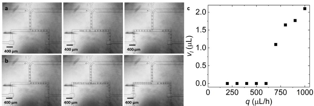
**Figure S2:** Drop sorting. Time lapse optical microscopy images illustrating the change in the flow direction of drops if the total injection speed is (a) 600  $\mu\text{L/h}$  and (b) 900  $\mu\text{L/h}$ . (c) The amount of fluid lost during the switching process ( $v_l$ ), as a function of the injection flow rate,  $q$ , is shown.
