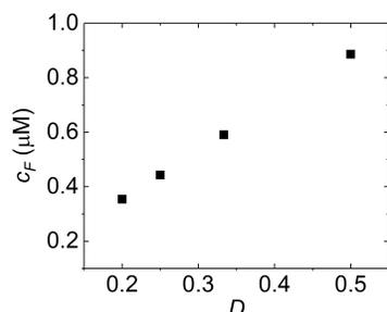
**Figure S1:** Influence of the duty cycle ( $D$ ) on the concentration of fluoresceine,  $c_F$ , contained in drops.
