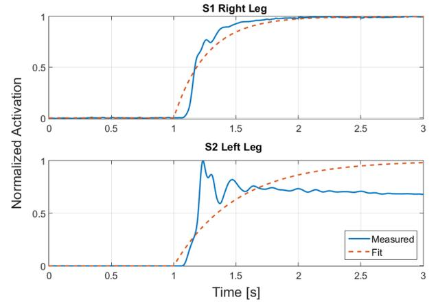
Figure 5: Muscle activation time constant results from parameter Test 3 for both participants. The normalized load cell data were used to determine the muscle activation time constant. The first order system time constant was found by a response that best fits the normalized measured data.
