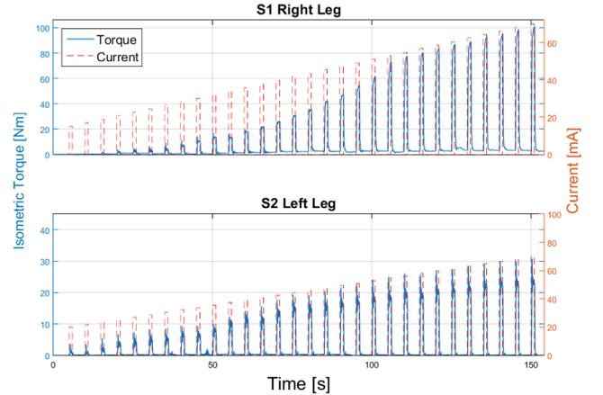
Figure 2: The results from parameter Test 1 for both participants. Stimulation current amplitude ramp to determine the threshold current amplitude,  $I_t$ , and saturation current amplitude,  $I_s$  of the participant. The threshold is the current amplitude that causes the first significant torque measurement, and the saturation is the current amplitude that produced the last significant change in the torque measurement.
