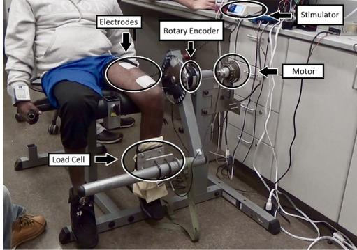
Figure 1: The modified hybrid neuroprosthesis system that combines FES quadriceps muscle with an electric motor.
