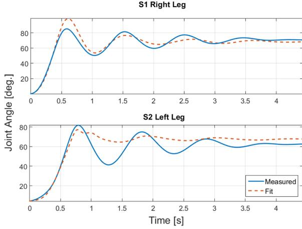
Figure 6: The results from parameter Test 4 for both participants. Plot of the results of the pendulum test with the response of the model that best fits the measured response.
