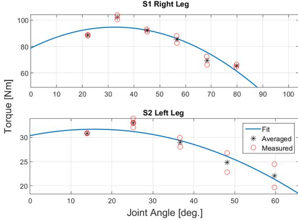
Figure 4: The results from parameter Test 3 for both participants. Torques produced during isometric contraction tests at different anatomical joint angles ( $\phi$ ), and the best fit of the measured data to find the torque-angle characteristics given in (3).
