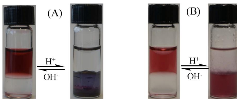
Figure S5. Control experiment to show that octadecylamine (ODA) facilitates the phase transfer of AuNP-MUA. (A) Photographs of glass vials containing aqueous solutions (top) of AuNP-MUA in contact with chloroform (bottom) without adding ODA. The initial aqueous solution of the AuNP-MUA in the vial was red in colour with pH > 4.1 (left). By adding 0.1 M HCl, the pH of the AuNPs aqueous solution was gradually decreased below 4.1 (right). After vigorous shaking and storing for about 2 min, the thin film of aggregated AuNPs, formed at water–chloroform and chloroform–glass wall interfaces. Re-dispersion of the AuNPs back to the aqueous phase is observed by adjusting the pH of the aqueous medium to > 4.1, by adding 0.1 M NaOH. (B) Photographs show the pH-triggered reversible phase transfer of AuNP-MUA between water and CHCl 3 layers with ODA, by switching the pH. The left side vial contains well-dispersed AuNP-MUA in an aqueous phase (top layer) at basic pH, and the right side vial contains AuNP-MUA transferred into the CHCl 3 phase (bottom layer), after adding HCl and vigorous shaking and storing for about 2 min.
