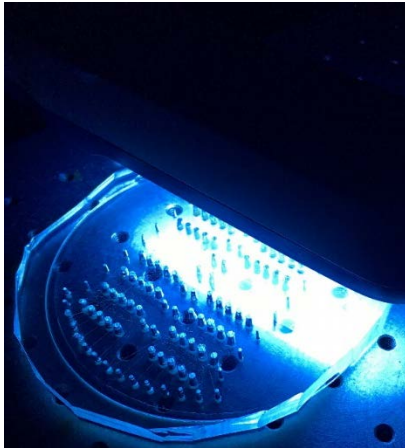
Figure S1. (a) Incubation of reporter tag, probe A, UV-cleavable probe, and Ebola RNA spiked blood on-chip at 50 °C. (b) Adding streptavidin beads into the incubation reservoirs. (c) After washes, Ebola targets released from beads with UVB exposure. (d) Fluorescence measurements.
