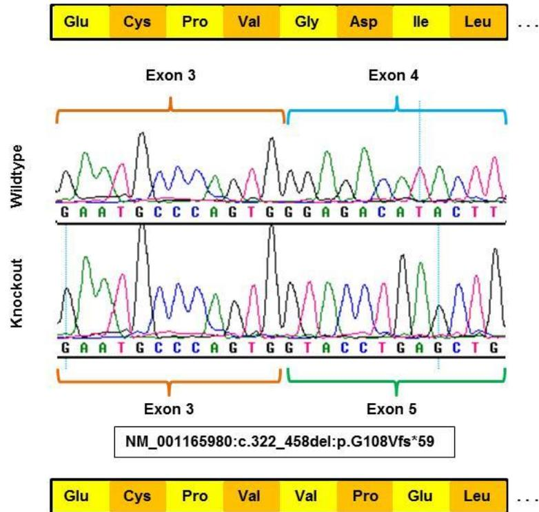
**Figure S3: DNA chromatogram of reverse transcriptase (RT)-PCR sequence, performed on the *Dcaf17* transcript fragment from the *Dcaf17* KO mouse and a wild type mouse for comparison.** Sequence data for the KO mouse reveals complete exclusion of exon 4 resulting in frameshift mutation (NM\_001165980.1:c.322\_458del:p.G108Vfs\*59) with concomitant premature stop codon after 59 residues. The corresponding codons are given as alternating yellow and orange boxes.
