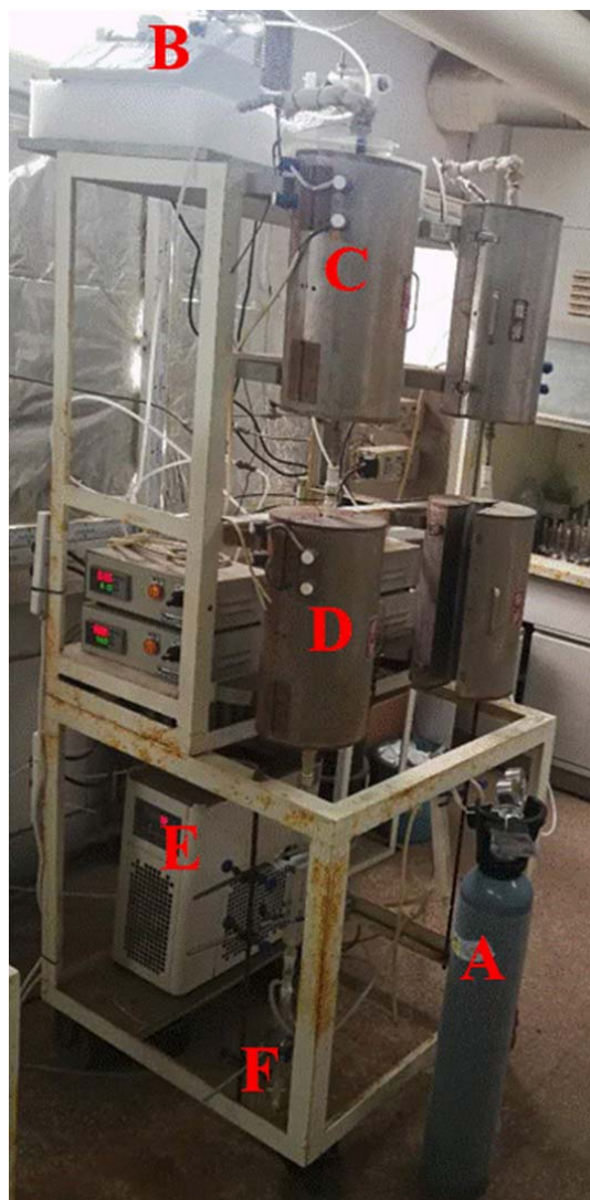
Figure R2: The flow reactor operation (oxygen canister (A), injection pump (B),
