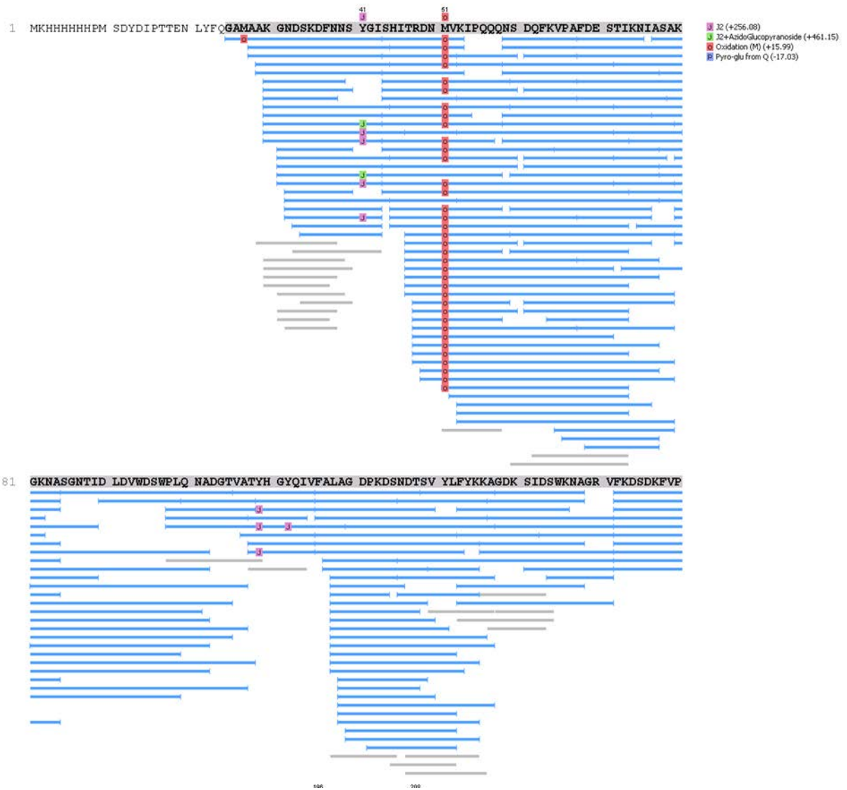
Supporting Figure 7. NanoLC-MS/MS analysis of elastase digested Y247F-2-1AzGlc. The enzyme was modified with 2 over 22 h. Modifier 2 is referred to as J2 in the picture. Supporting Figure 7 continues in the next page
