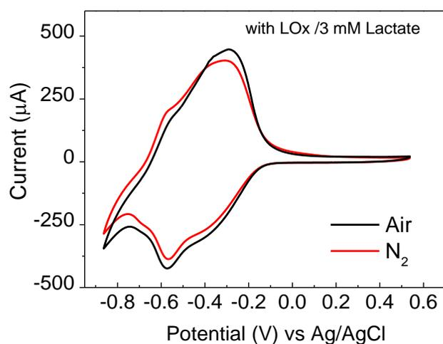
**fig. S9. The effect of air on the reaction of lactate with LOx-functionalized P-90.** CV curve of the P-90 film in air (black) and  $\text{N}_2$  (red) saturated PBS solution. The solution includes LOx and 3 mM of lactate.
