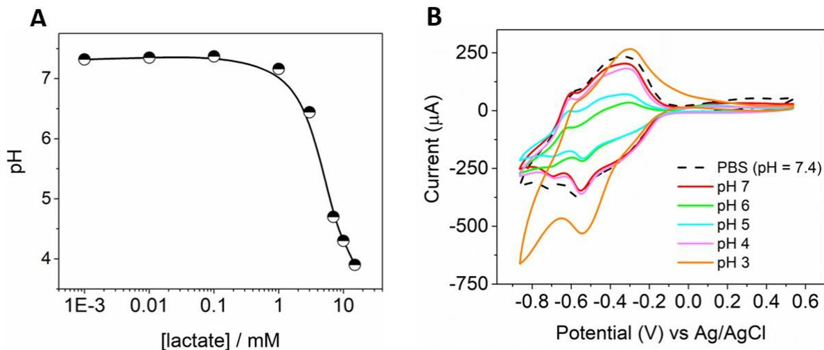
**fig. S7. The effect of pH on the CV curve of the P-90 film.** (A) The change in pH of the solution containing LOx as a function of lactate concentration, (B) the CV curves of P-90 film recorded in solutions of different pH.
