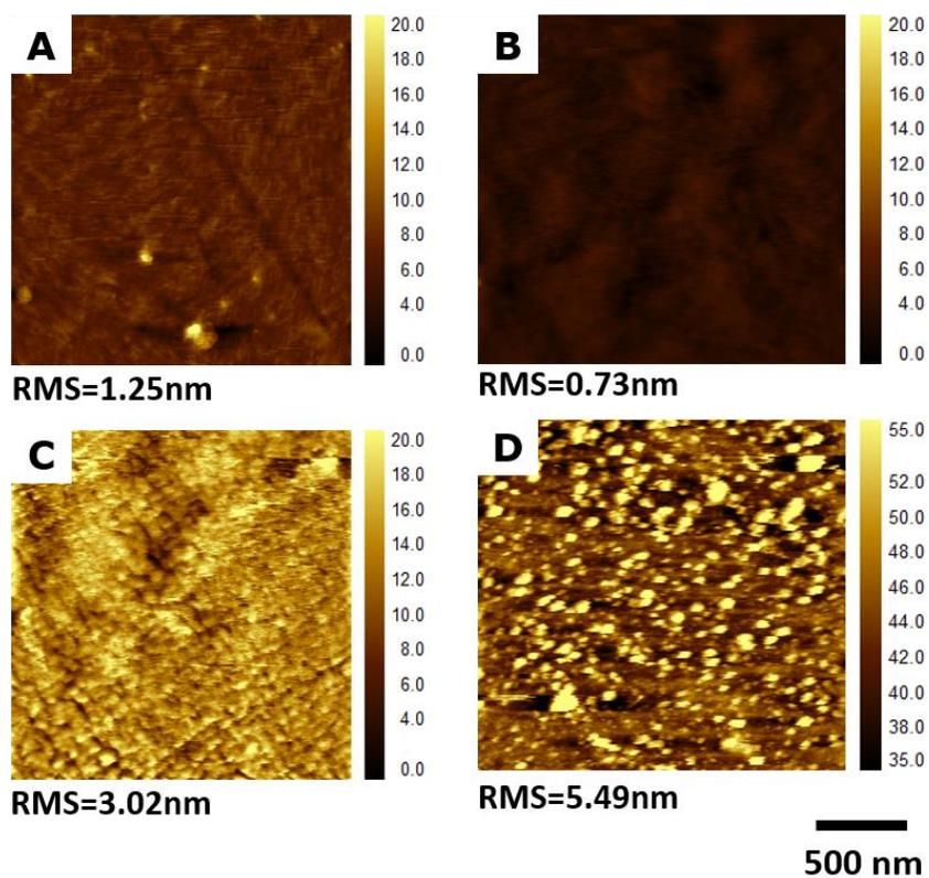
**fig. S5.** AFM topography images of the P-90 film coated on Au substrate. (A) in air, (B) immersed in PBS and (C) exposed to LOx, as well as (D) rinsed with PBS solution upon the incubation with the enzyme.
