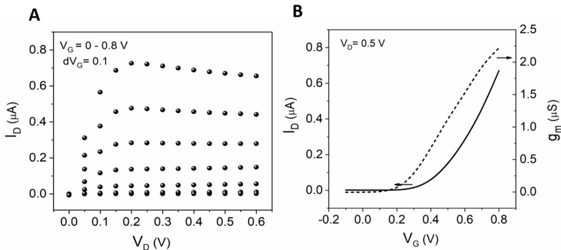
**fig. S1. The output and transfer characteristics of a typical all n-type polymer (P-90)-based OEET.** The corresponding transconductance values ( $g_m$ ) are shown in (B) along with the transfer curve ( $V_D=0.5$  V). The channel has a thickness, width and length of ca. 100 nm, 100  $\mu\text{m}$  and 10  $\mu\text{m}$ , respectively. The electrolyte is PBS.
