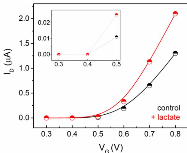
**fig. S2. Transfer curves of the OEET in the absence and presence of the enzymatic reaction.** The curves show the increase in  $I_D$  as a function of  $V_G$  ( $V_D=0.5$  V) in the presence (red line) and absence (black line) of lactate in the solution containing LOx. The onset  $V_G$  that needs to be applied for sensing lactate corresponds to the actual onset voltage of the device. The inset shows the magnified response of the device at low  $V_G$ .
