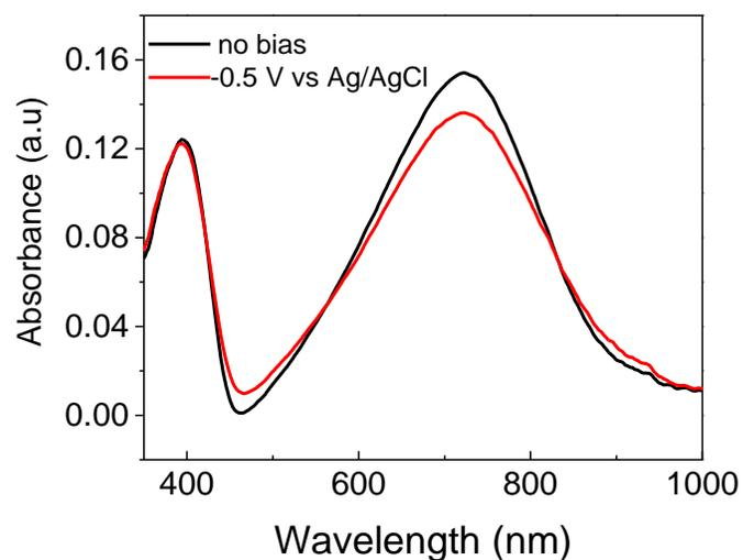
**fig. S8. The changes in the absorbance spectrum of the P-90 film during the electrochemical switch.** The absorbance spectrum of the film coated on an ITO substrate measured in PBS with and without applied bias (-0.5V vs Ag/AgCl).
