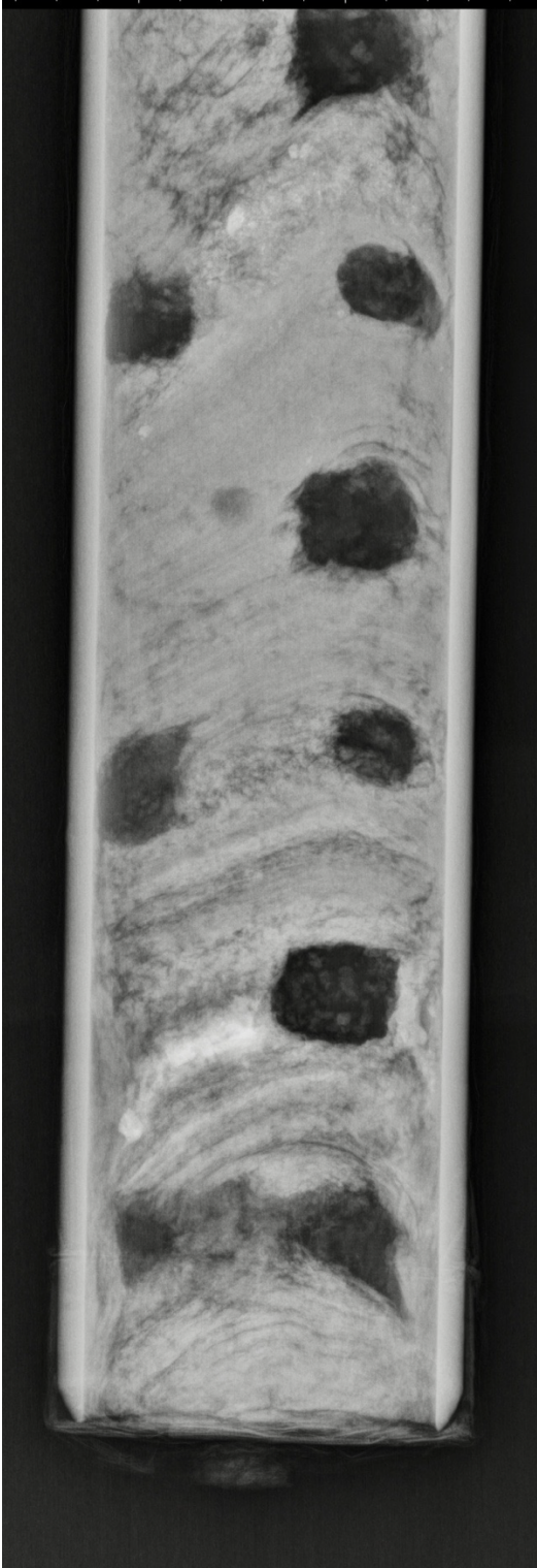
Fig. S1. X-radiograph of sampled basal sediments of core 14WLL-2A, demonstrating the laminated nature of the deepest LIG sediments (dark areas disrupting the stratigraphy are holes created by sampling).
