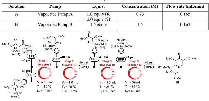
Table S3. Solution concentration and flow rates for the synthesis of 16.
