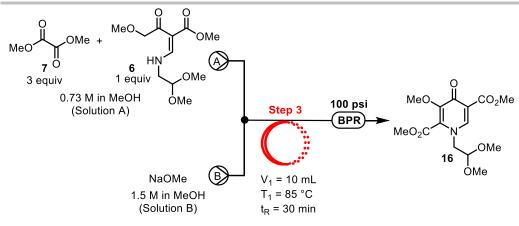
**Dimethyl 1-(2,2-dimethoxyethyl)-3-methoxy-4-oxo-1,4-dihydropyridine-2,5-dicarboxylate 16:** The Vapourtec R series flow reactor equipment consisting of two Knauer type HPLC pumps for reagent/solvent delivery and a 10 mL PFA reactor (1/16" O.D. x 0.04" I.D.) was utilized in the flow chemistry experiment. Before the start of the actual experiment, the reactor was primed with HPLC grade methanol.
