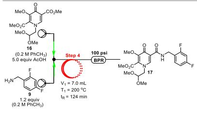
**Methyl 5-((2,4-difluorobenzyl)carbamoyl)-1-(2,2-dimethoxyethyl)-3-methoxy-4-oxo-1,4-dihydropyridine-2-carboxylate 17:** Flow setup was assembled with a 0.05" thru T-mixer (1/8" PEEK) at the entry to the reactor which consisted of stainless steel tubing 1/16" x 0.04" x 25'. Two solutions were prepared in 10 mL vials, and 7 mL of the resulting solutions were loaded into dry stainless steel Harvard syringes. Zaiput BPR was set at 100 psi, with the output directly going into a vial.
