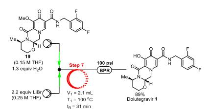
**pyrido**[1',2':4,5]**pyrazino**[2,1-b][1,3]**oxazine-9-carboxamide 1:** Flow setup was assembled with a 0.06" thru Tmixer at the entry to the reactor which consisted of PFA tubing 1/16" x 0.02" x 20'. Two solutions were prepared in 10 mL vials, and 6 mL of the resulting solutions were loaded into dry stainless steel Harvard syringes.
