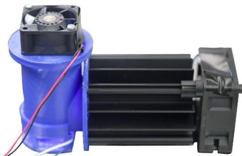
**Figure S9.** A photograph of the photoreactor with 365nm LED turned on and 0.5 dram vial holder attached.
