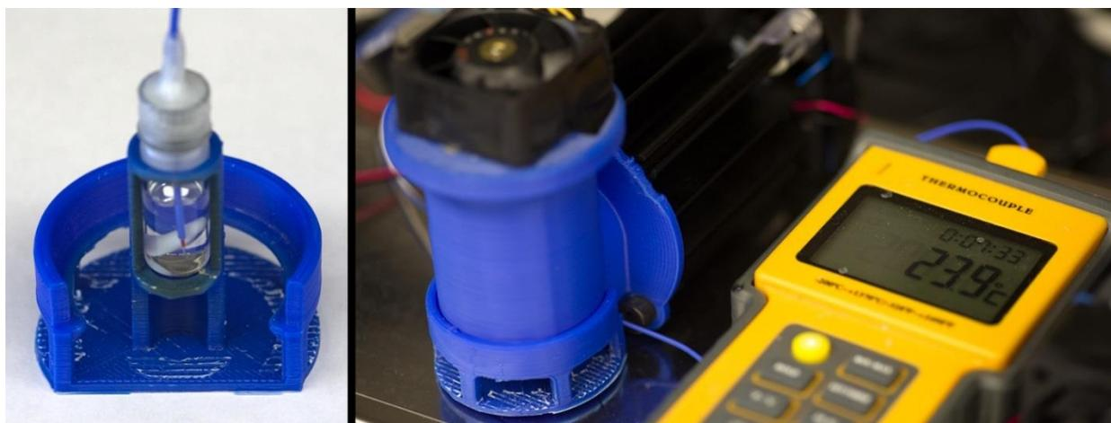
**Figure S11.** Temperature Monitoring Setup. A 0.5 dram vial equipped with a stir bar and 1 mL DMAc was monitored via a type K thermocouple inserted through the septum (**left**) and sealed with Parafilm. The vial was placed in the photoreactor as shown (**right**) and irradiated for 3 hours. The photo shown is before irradiation.
