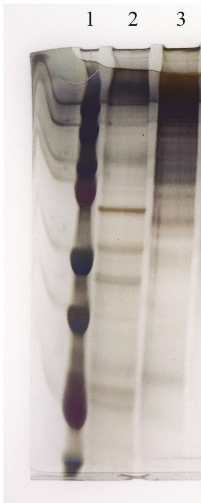
Fig. S6: Full length image of the SDS-PAGE gel shown in Figure 6. Lane 1 is loaded with the Precision Plus Protein Dual Color Standard. Lane 2 is loaded with 10 \mu\text{g} of the native pancreas from the same donor as Lane 3, loaded with 10 \mu\text{g} of decellularized pancreatic ECM. The remaining lanes of the gel contained samples unrelated to this project. The image shown in Figure 6a was cropped slightly to remove the edges of the gel, and rotated slightly to straighten the lanes.
