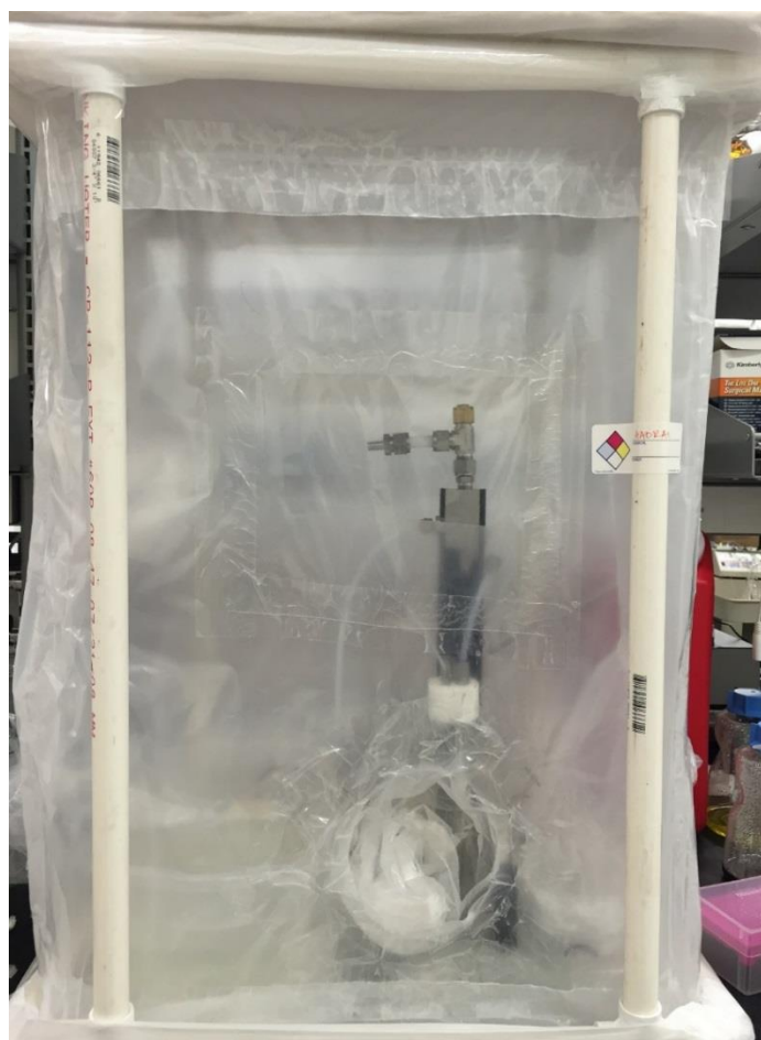
Figure S20. Photo of the commercial atomizer contained in a homemade humidity chamber.
