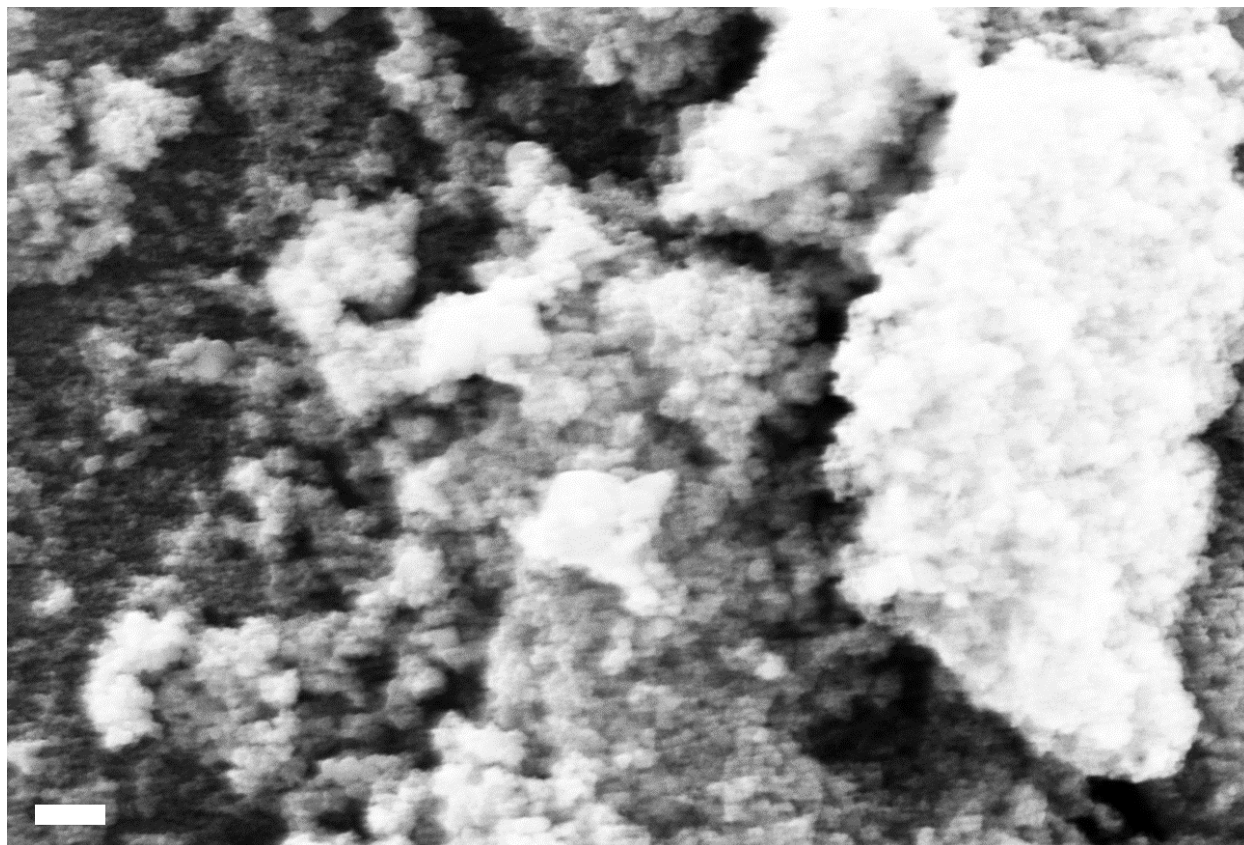
Supplementary Figure 12. SEM image of Fe 3 O 4 particles. Scale bar = 200 nm.
