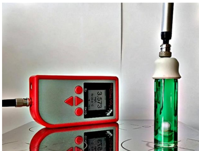
Figure S15: Setup of the in situ oxygen monitoring for a typical, not externally degassed Cu(0)-mediated RDRP.
