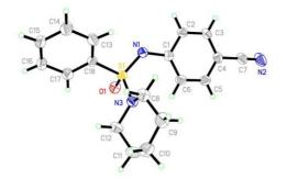
Compound **2bj** was crystallized by slow evaporation of a DCM solution of the compound at RT. A single crystal with dimensions of  $0.72 \times 0.15 \times 0.03 \text{ mm}^3$  was mounted on a CryoLoop using a protective oil. **2bj** crystallizes in the monoclinic space group *C2/c* with cell constants of *a* = 27.3860(14) Å, *b* = 7.8635(4) Å, *c* = 19.710(1) Å and  $\beta$  = 129.787(1)°. A total of 31481 reflections
