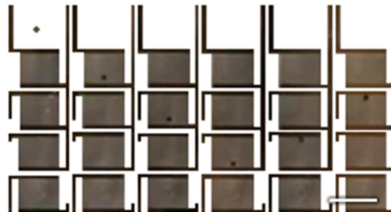
68 69 Supplementary Figure 9. Sub-nanoliter droplet manipulation using digital acoustofluidics. The 70 operating parameters for the IDTs ( e.g. , frequency, dimensions, and spacing) are optimized. The 71 droplets are generated using a T-junction in a conventional microfluidic chip and then are re- 72 injected onto the carrier oil. The measured volume of the droplet is 624 pL. The scale bar is 0.8 73 mm.
