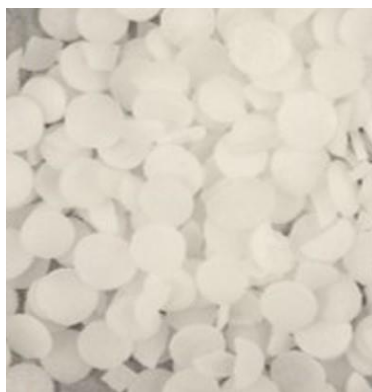
Figure S2 A digital photo of the TPP reagents, showing that the TPP are prone to form flake-like crystals.
