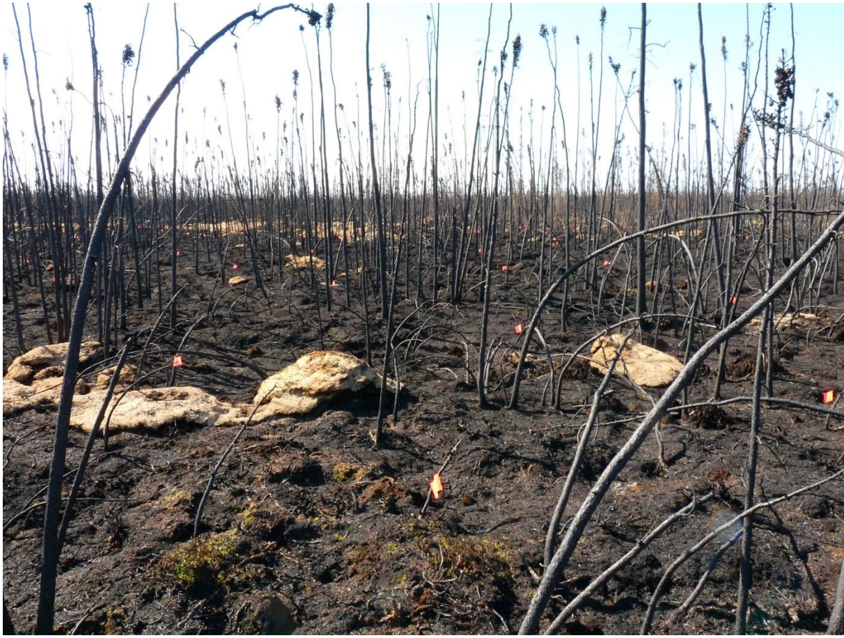
Supplementary Fig. 1. Soil thermal regime monitoring at the Kakisa burned peat plateau site (Supplementary Table 1). The site burned in 2014, two years prior to the study. Each peat plateau site had a 3 m spaced grid with 100 point locations marked with flags where depth to frost table was measured.
