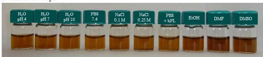
Figure S2. Optical images of ND-PEG-tNCIOs dispersed in (from left to right respectively) H 2 O (pH 4, 7, 10), PBS pH 7.4, NaCl (0.1, 0.15 M), PBS + hPL, EtOH, DMF and DMSO. (A) Freshly prepared solutions and (B) Solutions after 10 days.
