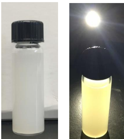
Supplementary Figure 1 | Digital images of PSS-IL dispersed in THF. (left) under natural lighting and (right) under flashlight.
