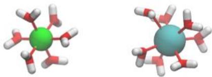
Figure S1. Structures of \text{Mg}^{2+}(\text{H}_2\text{O})_6 and \text{Ca}^{2+}(\text{H}_2\text{O})_7 . The structures were optimized using B3LYP/6-311++G(2d,2p)/PCM. The ion-water interaction energies calculated by RI-MP2/def2-QZVPPD are -336.67 and -264.38 kcal/mol for \text{Mg}^{2+} and \text{Ca}^{2+} , respectively.
