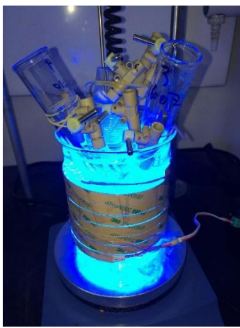
Figure S23. Stop-flow setup for fluorinated styrene screening and preparation.
