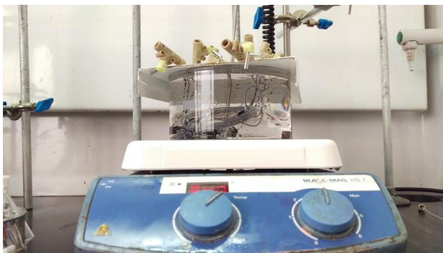
Step 9 : The SFMT reactors are moved to an off-line heating bath with desired temperature.
