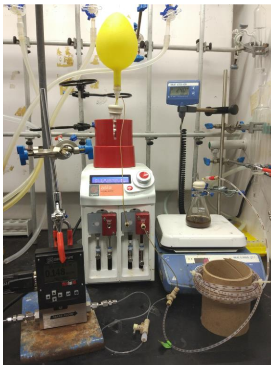
Figure S16. Continuous-flow setup for Sonogashira coupling with acetylene.
