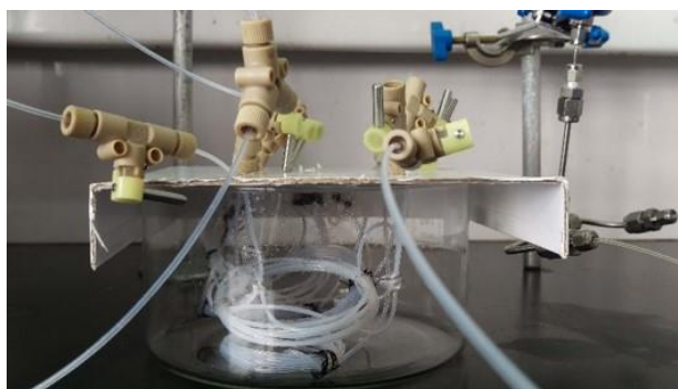
Figure S4. A close look at the SFMT parallel reactors.
