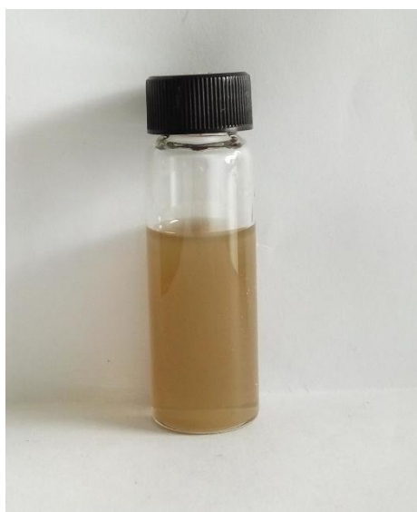
Figure S5. The supernatant of BP NSs dispersing in NMP obtained after centrifugation.
