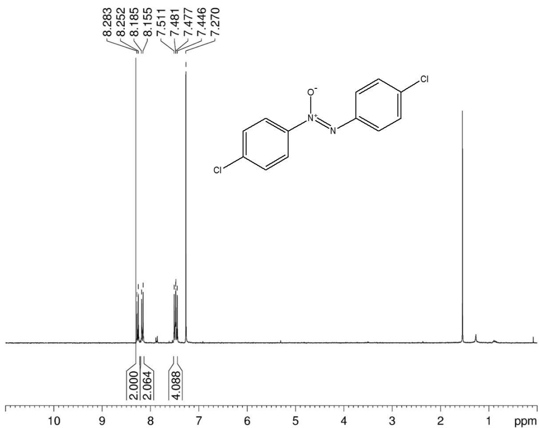
Supplementary Figure 24 | ^1\text{H} NMR spectrum of 4,4'-dichloride azoxybenzene. The residual solvent peak was used as an internal reference: ^1\text{H} (chloroform, 300 MHz). \delta 7.45–7.51 (m, 4 H, ArH), 8.15–8.19 (d, 2 H, ArH), 8.25–8.28 (d, 2 H, ArH)
