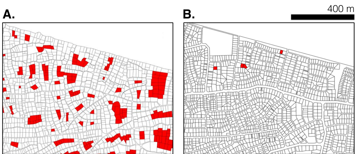
Fig. S6. Epworth (Harare, Zimbabwe) before and after reblocking. A Many blocks in Epworth in their original layout before reblocking. B The planned outcome of the re-blocking procedure proposed by the resident community. Parcels highlighted (red) do not have direct road access. This community-driven re-blocking process has created access to the vast majority of internal parcels.
