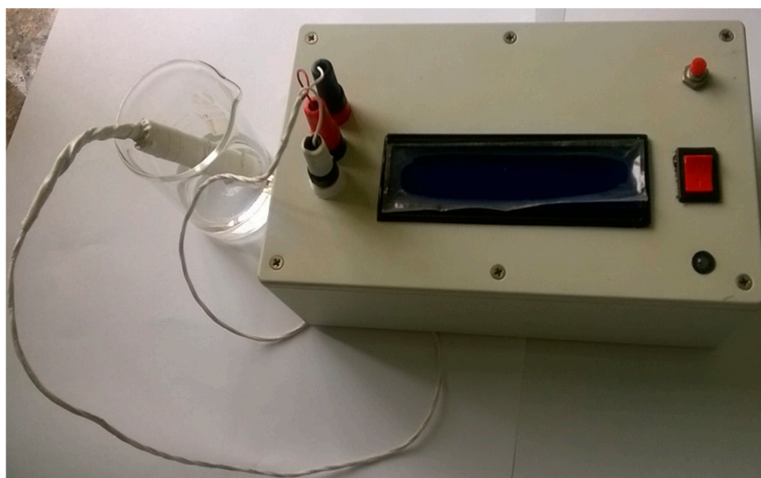
Figure S1. The image of the assembled portable electrochemical immunosensor designed for the on-site detection of aflatoxins.
