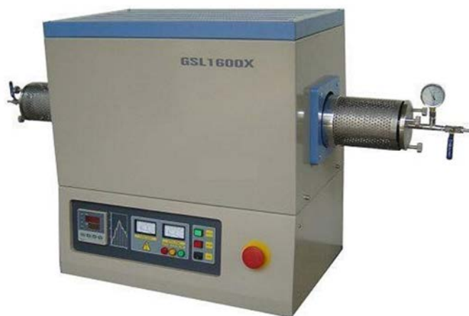
Figure S3. The picture of the atmosphere protection tube furnace in the experimental process.
