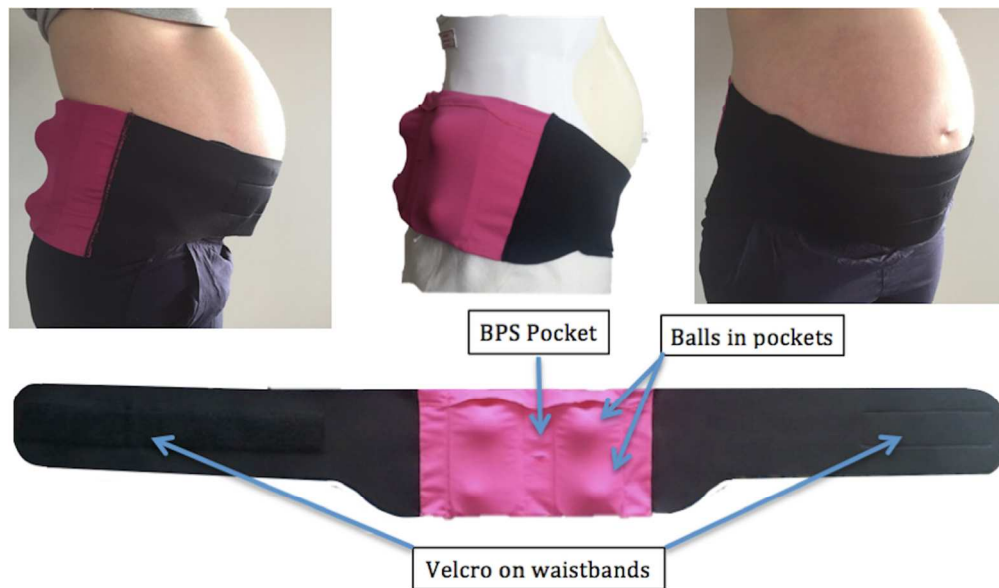
Fig. 1. PrenaBelt; BPS = Body Position Sensor.
