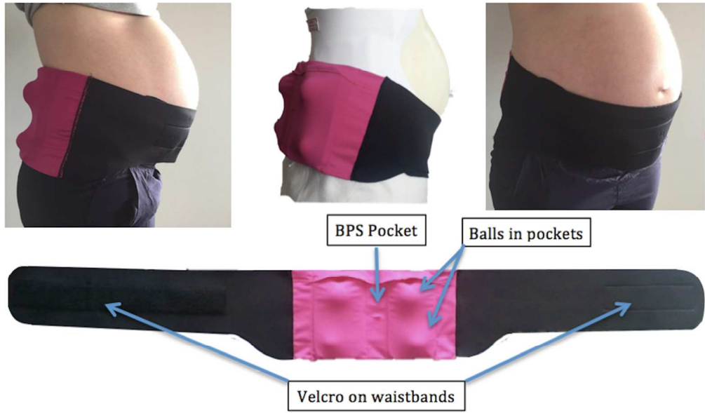
Fig. 1. PrenaBelt; BPS = Body Position Sensor.
