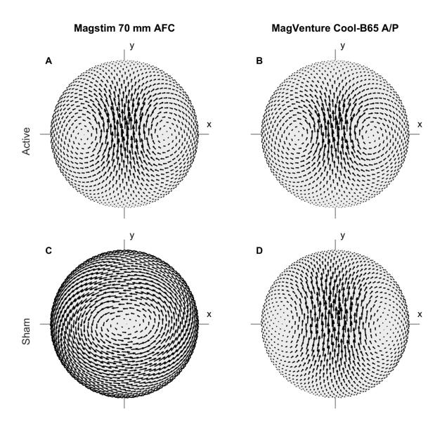
**Figure S1.** Measured E-field distributions for the active and sham coil configurations. Similar to figure 1A–D in the main text, but here the distribution for each coil is normalized by its maximum E-field strength.
