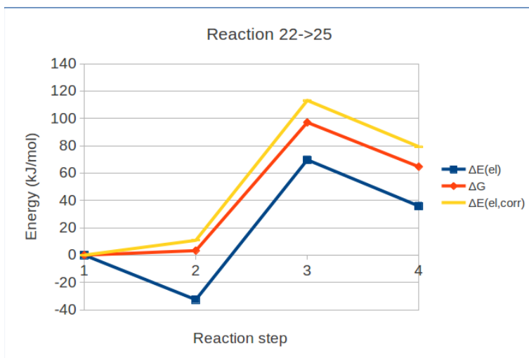
Figure S6: Reaction energy diagram of reaction 22 \rightarrow 25 showing the electronic ( \Delta E(\text{el}) ), Gibbs free ( \Delta G ) and electronic +43 kJ/mol ( \Delta E(\text{el,corr}) ) energy. The reaction steps are: 1) active site + gas phase methane, 2) active site + adsorbed methane, 3) TS of C-H bond dissociation, 4) active site + \text{CH}_3 group
