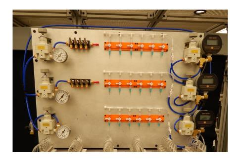
7. Finally, connect the whole filter assembly to a source of high pressure (>40 psi) air. House air or compressed air sources can be used. We typically mount to compressed air using a high pressure regulator connected to **Parts C** and **V** and then run **T1** from the filter assembly to the air source. Connections will vary based on your lab's air access.
