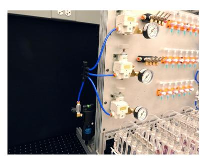
(!) Tip: We typically run tubing to air connections at the very end of all assemblies (shown by the completed control valve manifolds in the above image). This is an arbitrary decision; you can connect tubing at any time. We just find it helpful to do it all at once.
