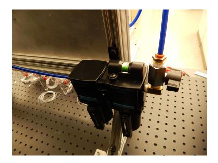
4. Create long segments of **T1 Tubing** to deliver compressed air to each regulator on both sides of the board using the 3-way push-to-connect manifolds (**Part T**) split. Connect the regulators to the 3-way push-to-connect manifolds on the left side as shown below.
