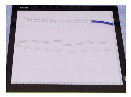
10. Attach the horizontal tubing segment to the elbow joint assemblies with **Tubing T2** connectors carefully.
