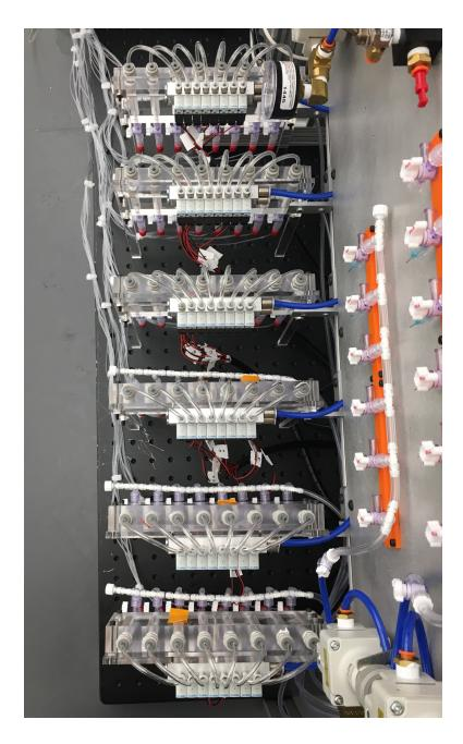
30. The completed setup for **Modules 1, 2,** and **3** should appear as the following image. Note the manifold connections for the 6 manifolds from the Control Switchbox from **Module 1**.
