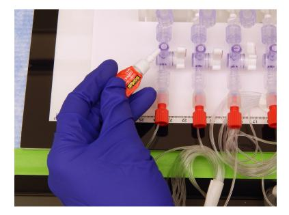
9. Assemble the horizontal tubing assembly according to the Module schematic as shown below. Use ~1" regular segments of **Tubing T2** to connect the T tube fittings (**Part K**). This is similar to the flow manifolds you assembled in **Module 1**. Attach an end cap (**Part L**). This assembly (loading port) will be attached to **Tubing T1** segments from the Control Loading module in **Module 4**.
