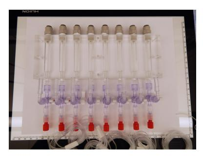
Align the stopcocks parallel to one another. Remove the barbed elbow assembly (Part c, Tubing T2) from the 4-way stopcock (Part N) and superglue the stopcock connectors to prevent leaks. It is important to perform this operation now, despite the disassembly, because it will ensure each stopcock is precisely aligned horizontally in space with the rest of the control loading assembly. Re-attach the elbow joint assemblies.
