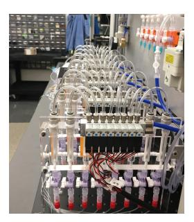
5. After **Module 5**, the valve wiring collections wired into the WAGO will appear like this image.
