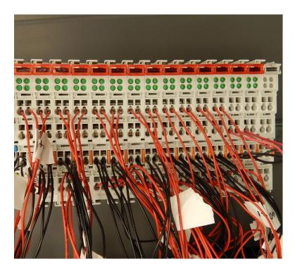
12. Wire the global ground wire (yellow wire from the ending input lane) to the first module of the I/O controller base (**Part W1**) as shown below. Insert the striped wire in the bottom right input of the module. This connects the input ground to the shared module
