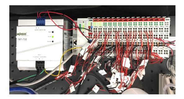
You should see the power lights and connectivity lights (**Parts W1, W2**) on in your setup upon powering the WAGO but valve state lights (top of **Parts W3**) may or may not be active yet depending on the initialization parameters.
