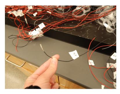
3. Cut ~14" pieces of **Tubing T5**. Collect all the solenoid wires from one manifold and gently snake the **T5 Tubing** up the collection of wires to organize and secure them This step tidies up the wires so that wiring the WAGO Modbus controller is easy and less messy.
