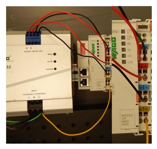
13. Next, connect the Ethernet cable, **Part m**, to the top Ethernet port (shown above) of the WAGO I/O (**Part W1**) and to your computer. Change the WAGO dipswitch (top red box on **Part W1**) to the desired WAGO Ethernet address. We use 192.168.1.3 but this address may depend on your institutional requirements. Use the manufacturer instructions to change the dipswitch as desired.
