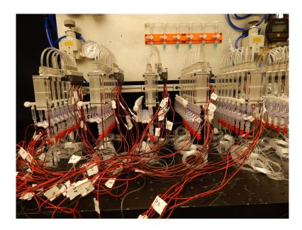
(!) Tip: It is important to label **both** the top and bottom wires with the valve number as we later will place black hosing around all the wires from one manifold to organize and secure them. Without the top labels, it becomes difficult to isolate individual valves connections if there arises a problem or if the setup must be dissembled (for moving around, for instance). Use a label maker or solvent resistant markers on lab tape when labelling the solenoids.
