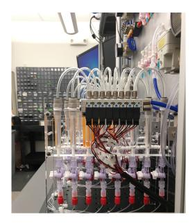
(!) Tip: Start from the bottom of the collection of wires, wrap the first end around the whole group, and thread the tubing upward by coiling to the right. Stop coiling when the tubing reaches the labels near the solenoid array. Be sure to keep labels at both the top and bottom of each wire visible. T5 should terminate tubing ~2" from valve solenoid arrays, as shown above.
