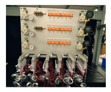
1. Each red and black wire set controls the positive voltage and ground connections, respectively, for each solenoid. Starting with the leftmost manifolds, label the top and bottom of the red and black wires associated with each solenoid valve with the valve number, starting at 0 (e.g. Manifold 1 = Valves 0-7, indexed per each red and black wire). Place the bottom label ~7" from the end of the wire (to make room for stripping
