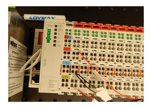
11. Repeat for Valves 2, 3 using the right breakouts for the first module then continue wiring all the rest of the valves. Your WAGO build should now look like this.
