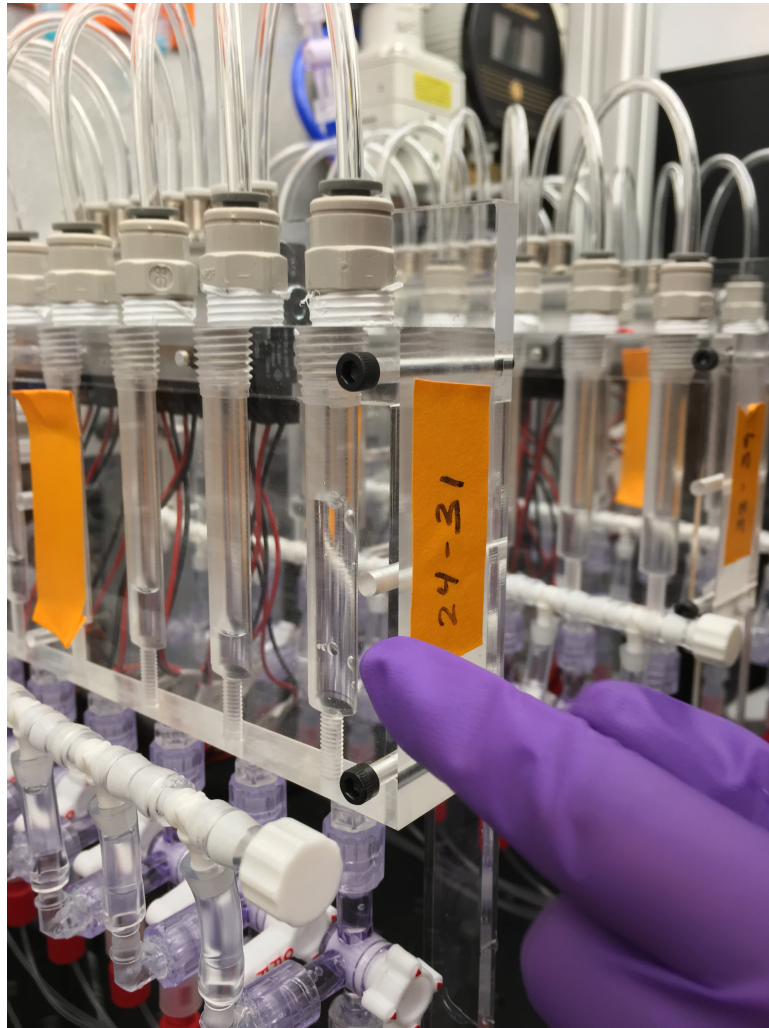
Water filling the reservoir for Valve 24.
