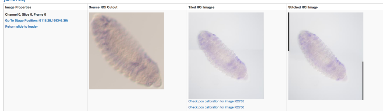
Figure S14. Summary report after acquisition, Related to Figure 1. Shown is a screenshot from the browser. Hyperlinks on the left allow for loading the slide and positioning at the location of the object. The images on the left are from low resolution (5x) phase 1, middle are composite of roughly tiled (according to coordinate position) high resolution phase 2 images (20x), and right composite images showing the result of the image stitching module.
