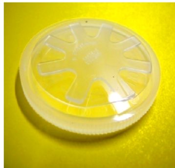
Fig. S24. GaN-based LED wafer prepared by MOCVD system (2").
