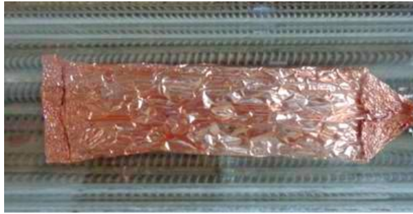
Fig. S6. Photograph of Cu pocket used for producing higher vapor pressure of Cu to protect the Cu NWs from melting under high reaction temperature.
