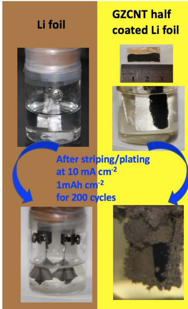
Supplementary Figure 14. In-situ observation of blank and GZCNT coated Li foil before and after Li stripping/plating. Li foil is half coated by GZCNT layer to clearly show its protection of Li anode from the dendrite formation. The electrolyte employed was 0.6 M lithium bis(trifluoromethanesulfonyl)imide and 0.4 M \text{LiNO}_3 in 1:1 w/w DOL/DME. The cells are charge/discharge at 10 \text{ mA cm}^{-2} with 1 \text{ mAh cm}^{-2} capacity for 200 cycles.
