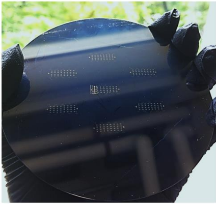
Fig. S17. Wafer-scale fabrication of the RF rectifier arrays. (a). the photograph showing the wafer scale RF rectifier arrays. (b). The performance of the rectifier at 50 MHz. Photo credit: Xiaoxue Wang, Massachusetts Institute of Technology
