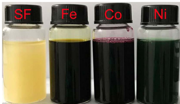
Supplementary Figure 1 | Photographs of the as-obtained typical regenerated silk fibroin solutions prepared by dissolving degummed natural silk using concentrated salt solution of NaCl, \text{FeCl}_3 \cdot 6\text{H}_2\text{O}/\text{ZnCl}_2 , \text{CoCl}_2 \cdot 6\text{H}_2\text{O}/\text{ZnCl}_2 , and \text{NiCl}_2 \cdot 6\text{H}_2\text{O}/\text{ZnCl}_2 , respectively.
