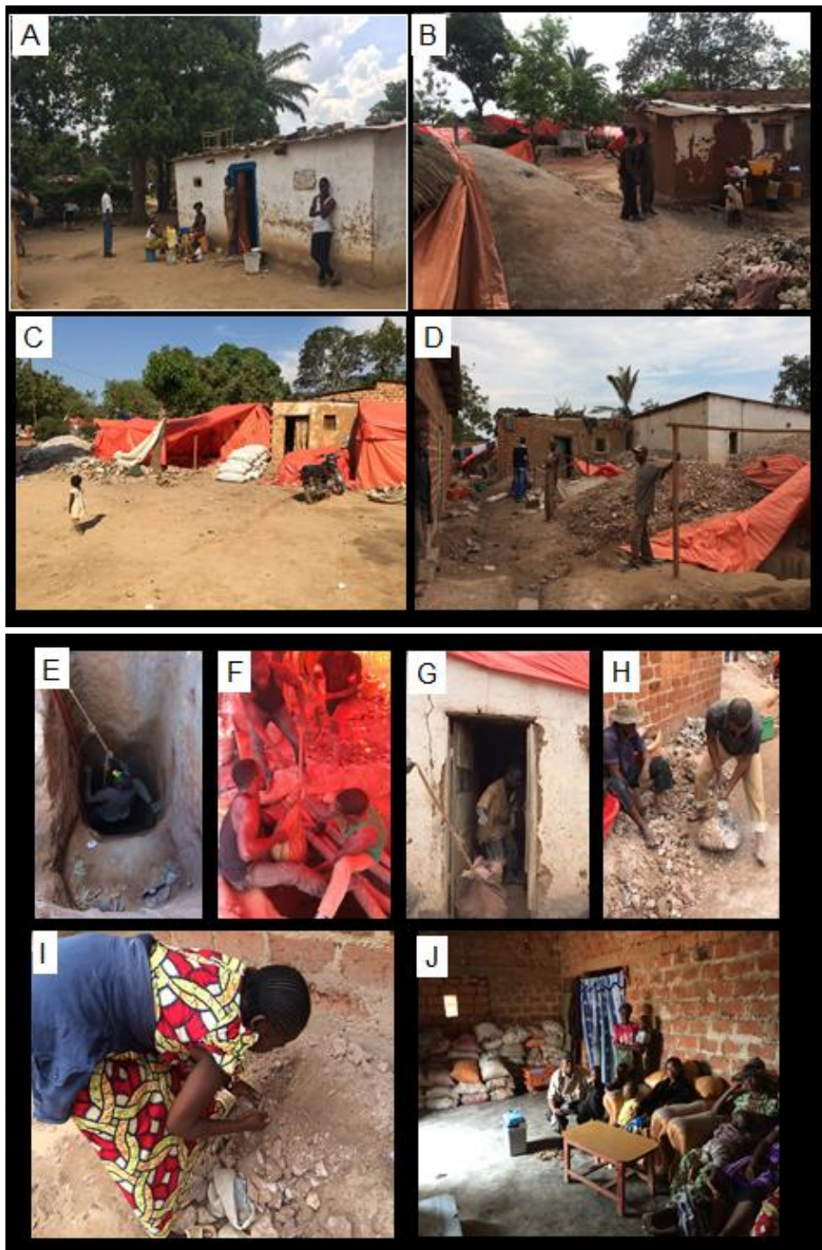
Photographs of a plot in the control area without mining (A) and of various plots in the mining area (B, C, D) showing the presence of numerous mine pits, covered by orange plastic sheeting, and mine tailings close to houses; a mineworker descending in a mine pit (E); mineworkers hoisting a bag of ore from a mine pit under plastic sheeting (F), and from a pit dug inside a house (G); mineworkers crushing blocks of ore containing black heterogenite (H); a woman collecting pieces of ore (I); a living room with bags of ore stored in the back of the room (J). Photographs D, H, I, and J were taken from the same plot. Letters do not correspond with codes of plots in Figure 1. (Photographs taken by B. Nemery, November 2014).
