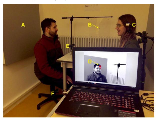
A: Homogeneous grey wall enhancing detection; B: Stand with calibration screen grid, swings towards nose with central point (arrow); C: Stand with Full HD Scene cam; D: Live view of scence cam with red dot indicating gaze point; E: Eye-tracker; F: height adjustable chair.
