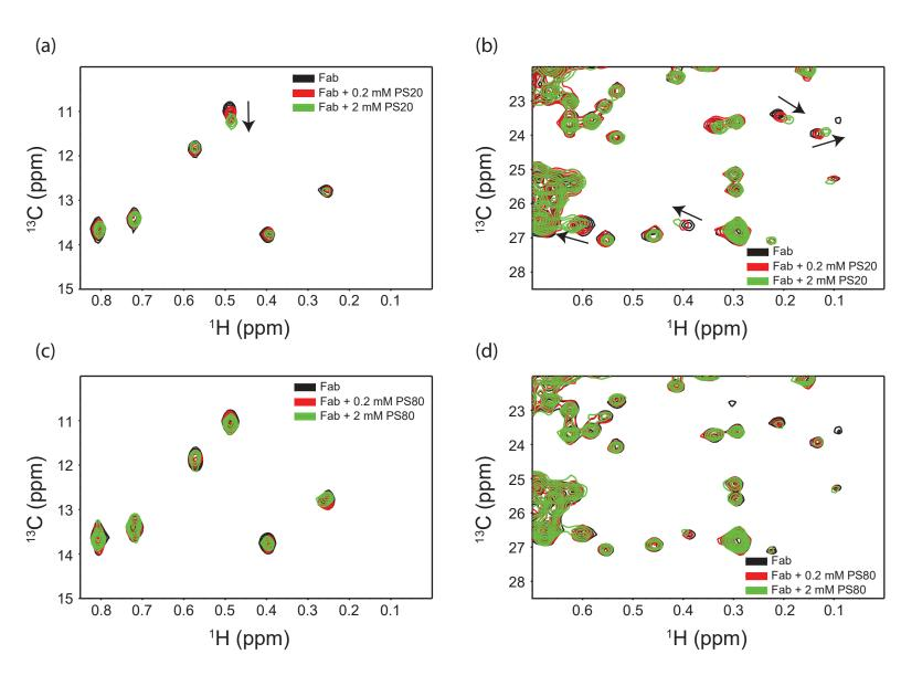
**Figure S3.** Addition of PS20 caused chemical shift changes in the Fab region compared to PS80.
