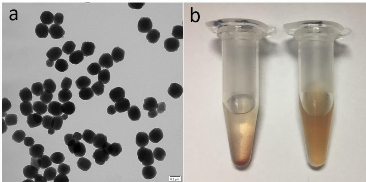
**Figure S6.** a) TEM of HfMOF nanoparticles. b) HfMOF nanoparticles before (left) and after phosphate-terminal aptamer conjugation (right) in water.
