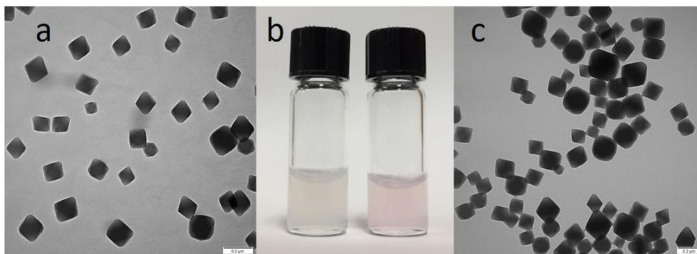
**Figure S5.** a) TEM of UiO-66 nanoparticles in DMF. b) Digital picture of UiO-66 nanoparticles before and after conjugation of phosphate-terminal aptamer modified with TAMRA (left: UiO-66 nanoparticles in DMF, right: UiO-66-aptamer in water). c) TEM of UiO-66 nanoparticles in water.
