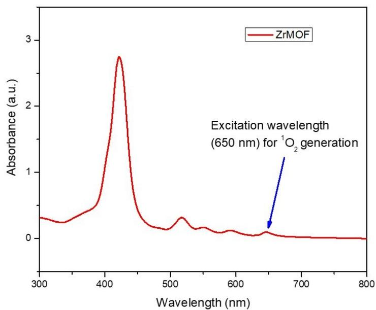
**Figure S4.** UV-Vis absorption of ZrMOF nanoparticles.
