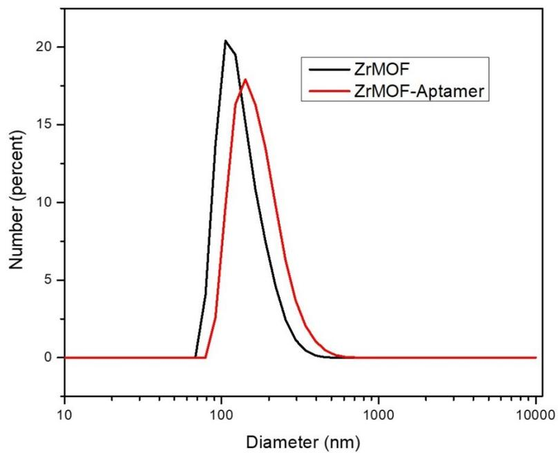
**Figure S2.** Dynamic light scattering of ZrMOF nanoparticles before and after phosphate-terminal aptamer conjugation.
