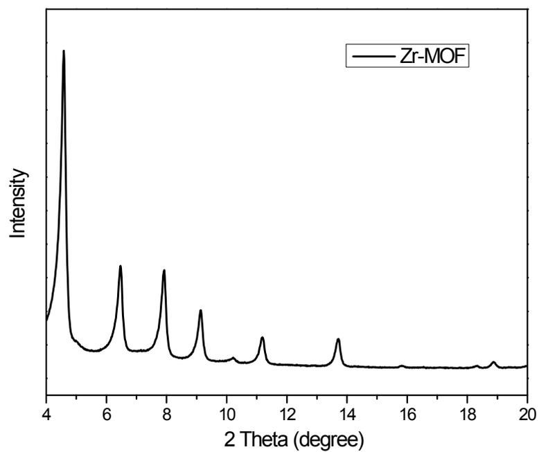
**Figure S1.** X-ray diffraction of as-synthesized ZrMOF nanoparticles.
