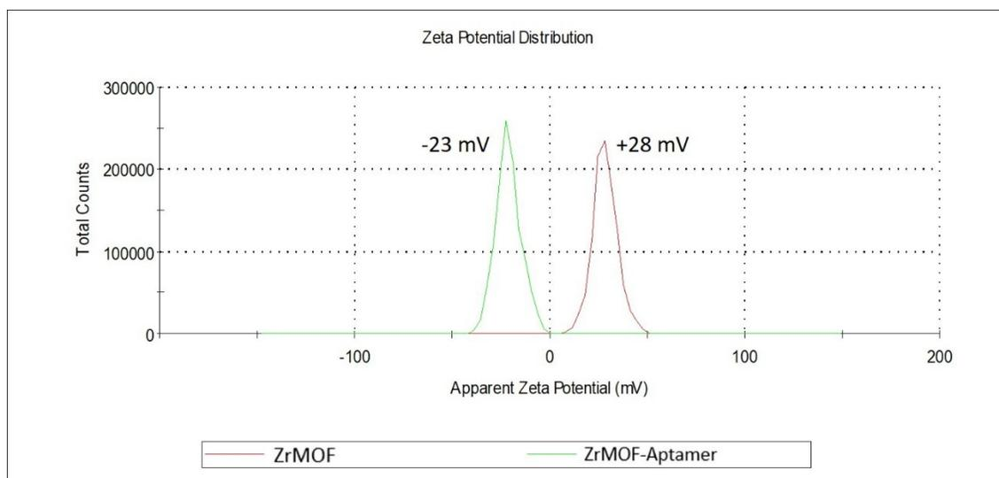
**Figure S3.** Zeta-potential of ZrMOF nanoparticles before (red) and after (green) conjugation with phosphate-terminal aptamer.
