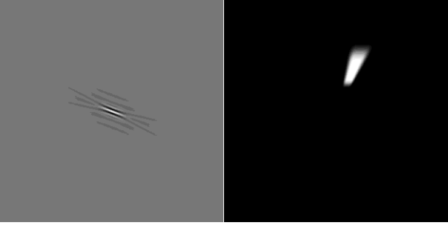
Fig. S1. An example of a curvelet (left) and its Fourier transform (right)
