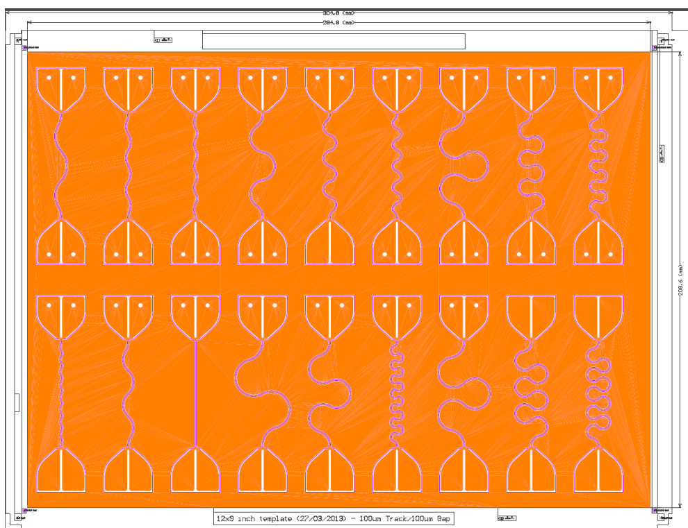
Figure S2. AutoCAD circuit design file for the meanders tested using the tensile tester.
