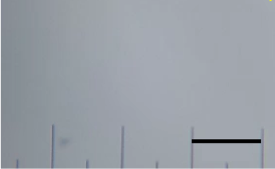
Supplementary Figure 10. Micrometer scale used for cellphone system calibration. The scale bar is 100 \mu\text{m} .
